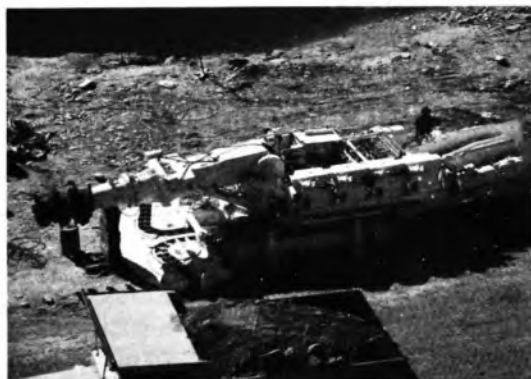
Photo 1: A view of the Road header
